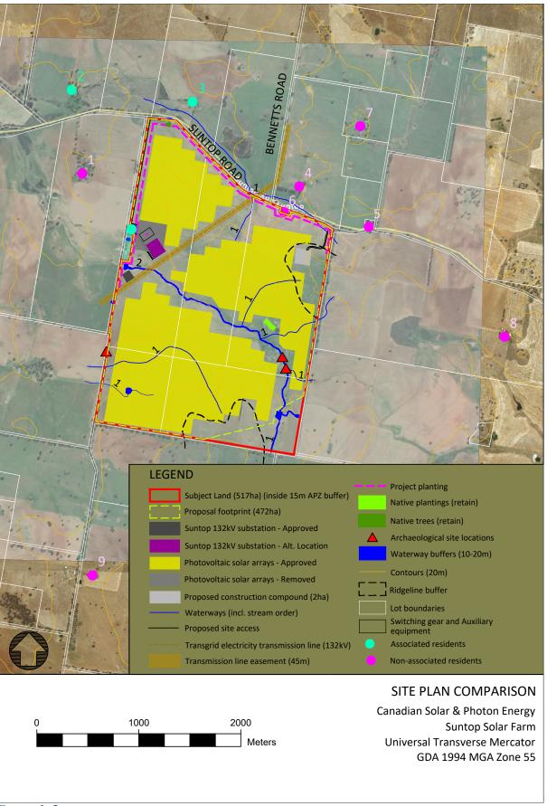
FIGURE 2: SITE LAYOUT PLAN SHOWING COMPARISON OF APPROVED AND PROPOSED SUBSTATION LOCATION
