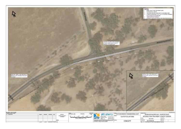
Figure 3. Proposed Widening of Renshaw - McGirr Way at the Suntop Road Intersection.
